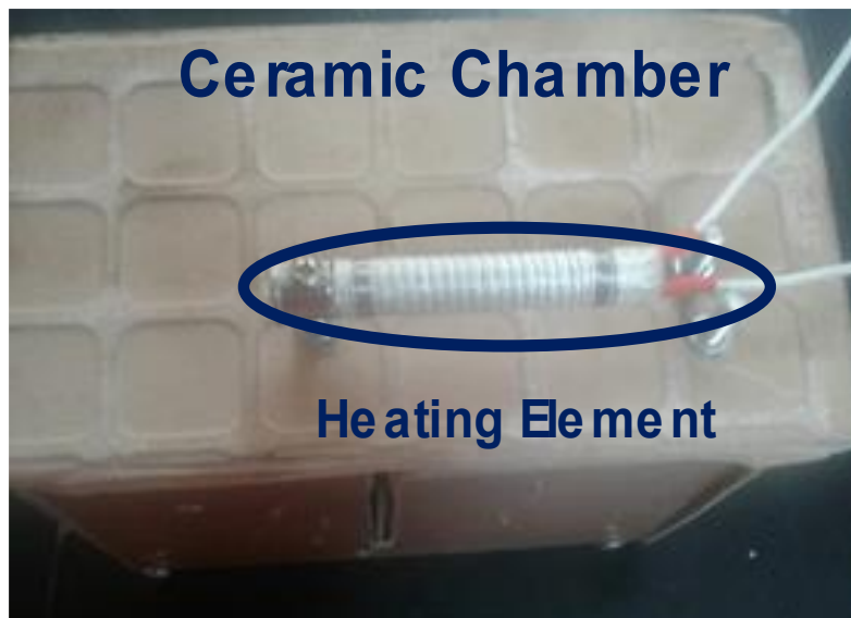
Figure 8: Heating chamber with the heating element
