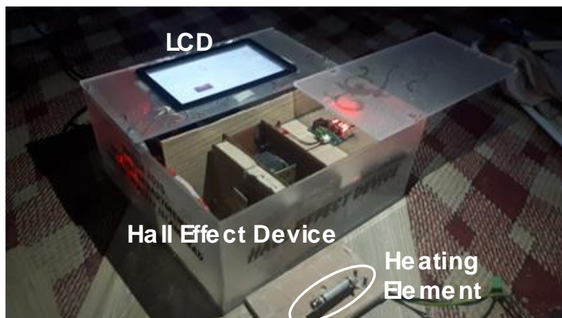
Figure 9: Hall Effect Automated device for temperature control
