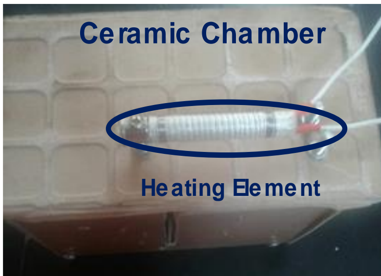
Figure 8: Heating chamber with the heating element
